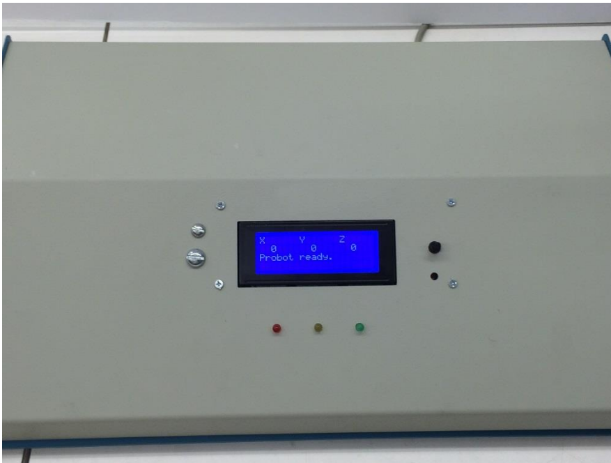
Figure 17: A Close Up on the Enclosure containing the server, controller, LCD, and power supply.
