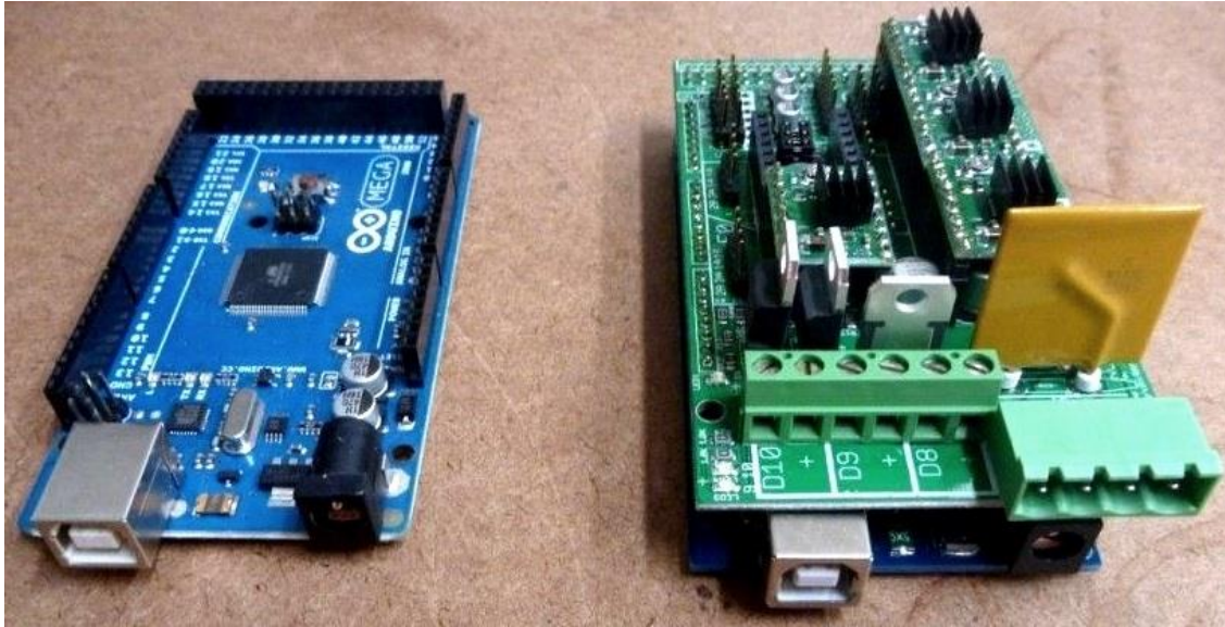
Figure 6: Arduino Mega 2560 with and without RAMPS 1.4 shield on top
