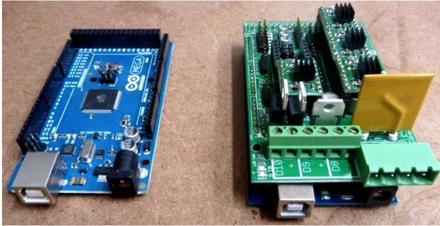
Figure 6: Arduino Mega 2560 with and without RAMPS 1.4 shield
